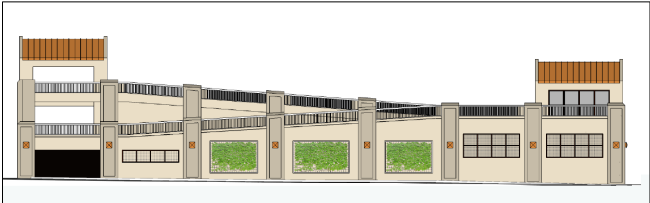
PARKING STRUCTURE: LAKESIDE AVENUE- ONE LEVEL BELOW GRADE/TWO LEVELS OF STRUCTURED PARKING:
